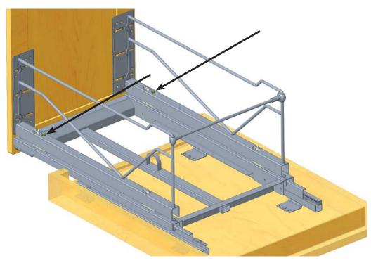
3. Remove the complete door-rail-unit (don't remove or loosen any door mounting screws)
