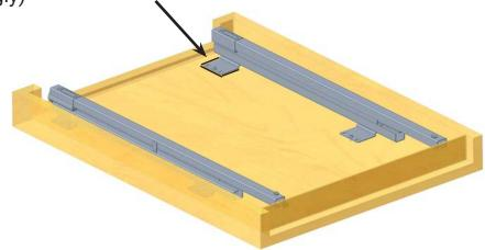
6. Assemble the unit in reverse order. While installing the bottom frame make sure it's hooked-in at the rear side. Place the door-rail-unit on top of the four ClickFixx bolts and move the door-unit against the bottom frame until the green bolts are locked
